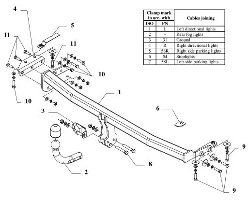
This towbar is designed to assembly in following cars: **NISSAN PRIMERA**, **4/5 doors**, **(P11)**, produced since 09.1996 till 08.1999, catalogue no. **V54** and is prepared to tow trailers max total weight **1700 kg** and max vertical load **75 kg**.
