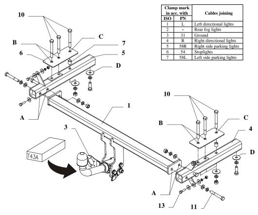
This towbar is designed to assembly in following car: **KIA CARENS I II, (FC, FJ) VAN** produced since 01.2000 till 08.2006, catalogue no. **T43** and is prepared to tow trailers max total weight **1250 kg** and max verticalload **75 kg**.
