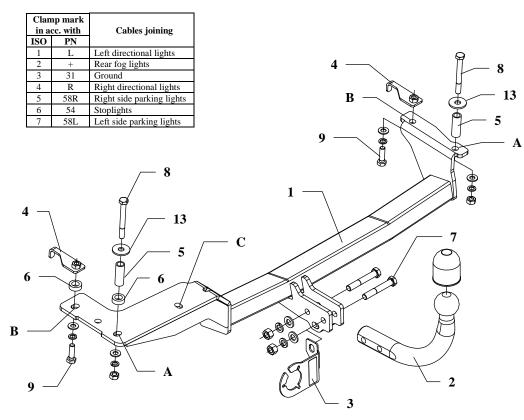
This towing hitch is designed to assembly in following cars: **SEAT IBIZA, 3/5 doors, (S03, 6K),** produced since 07.1993 till 01.1996, catalogue number **SC01** and is prepared to tow trailers max total weight **1100 kg** and max vertical load **75 kg**.
