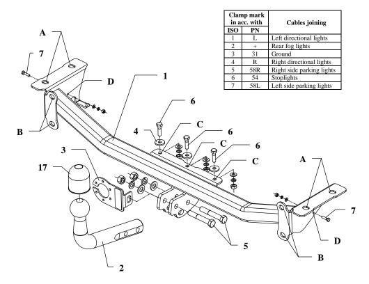
This towbar is designed to assembly in following car: **FIAT CINQUECENTO, 4 DOORS,** catalogue no. **S07,** produced since 1992 till 1998 and is prepared to tow trailers max total weight **400 kg** and max vertical load **28 kg**.
