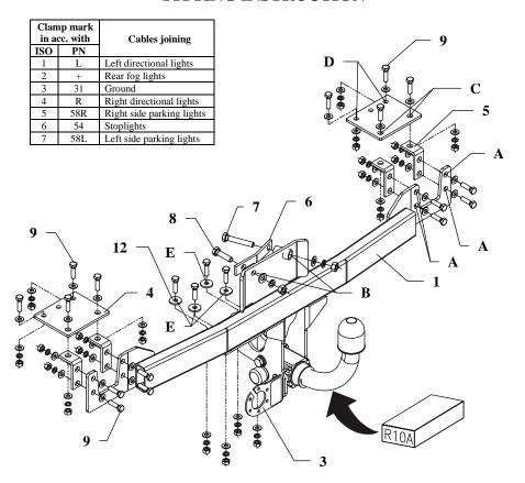
This towing hitch is designed to assembly in following cars: **FIAT BRAVO, 3 doors (182),** produced since 09.1995 till 10.2001, catalogue no. **R10A** and is prepared to tow trailers max total weight **1400** kg and max vertical load **75** kg.
