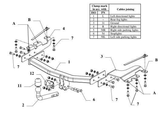
This towbar is designed to assembly in following cars:
