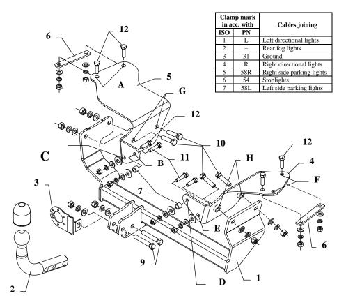
This towbar is designed to assembly in following cars: **ALFA ROMEO 147, 3/5 doors, except TI-Model, GTA3.2L 184KW** produced since 2000, catalogue no. **AL37** and is prepared to tow trailers max total weight **1300 kg** and max vertical load **60 kg**.
