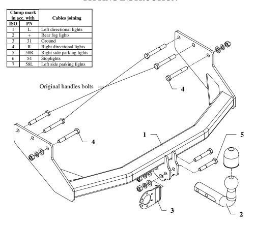
This towing hitch is designed to assembly in following cars: **FORD TRANSIT, metal build-up, also MAXI. loading platform,** produced since 11.1991 till 04.2000, catalogue no. **C18** and is prepared to tow trailers max total weight **2000 kg** and max vertical mass **75 kg**. Towbar is designed in way excluding diassemble, cut out or drill a bumper.
